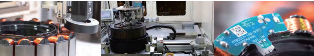
Automated production to boost productivity and yield. Data management with our QR Code system in each process step to ensure quality and traceability for every single product.
